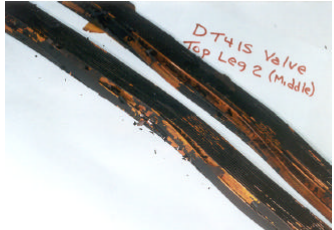
Fig. 5 February 2000 failure showing thermally degraded enamel on strands of Leg 2 valve winding at top of coil near static ring
